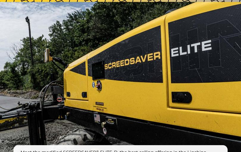
Meet the modified SCREEDSAVER® ELITE-D, the best-selling offering in the Ligchine SCREEDSAVER line of innovative, labor-saving machines. The SCREEDSAVER ELITE-D is loaded with features including all-wheel drive, heavy-duty boom reaching 18 feet and 33-gallon on-board fluid tank.
