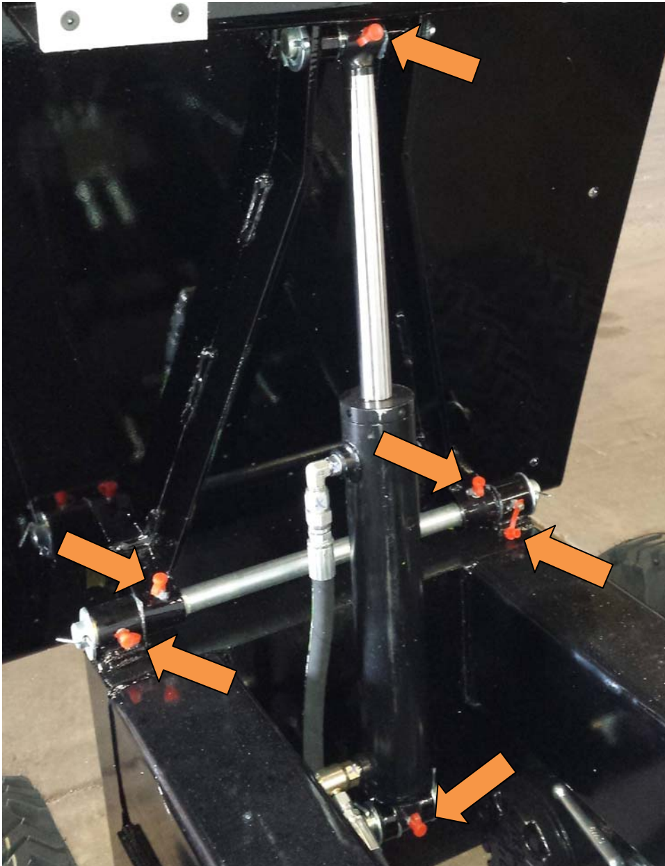
Figure 13: Dump box hinge and lift cylinder grease fittings
